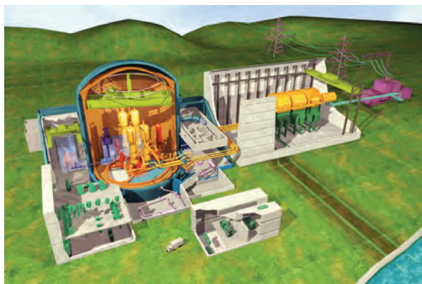
Figure 1. Schematics of nuclear island of EPR of 1.6 GWe, with turbine building and water cooling. No big hyperboloid cooling towers and scrubbers are necessary for the operation, but just a vast source of cooling water [11]. The small dimensions of the plant can be estimated by looking at the truck.
